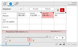
Configure all user-settable alarms (A. Low threshold, B. High threshold)
